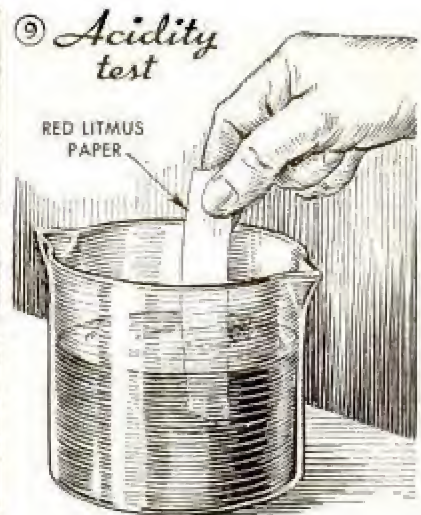
Red litmus paper immersed in soluble cutting oil should turn blue. If this does not happen, add soda ash to the oil, a little at a time, and stir in, testing with fresh red litmus paper between additions
